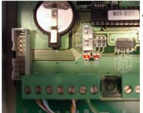
When blocking the receiver closest to the entrance, the red led A on the Minilogger should lit. If the B led is activated, switch the wires A and B.
