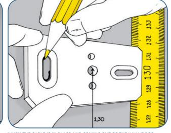
WHEN THE CABLE IS IN PLACE AND COMING OUT OF THE WALL/DOOR-FRAME, MARK THE POSITION FOR THE SENSORSET..
